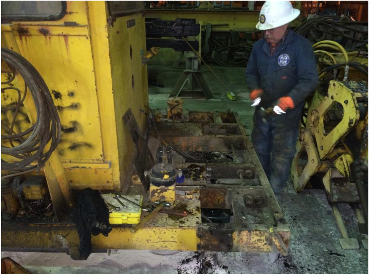
Mike pulls the last of the deck-plating. Conversion can begin. The regulator is dead. Long live the tug!
